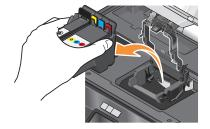
**Warning—Potential Damage:** Do not touch the printhead nozzles.
