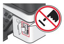
**Warning—Potential Damage:** Do not touch any cables, any network adapter, any connector, the USB Bluetooth adapter, or the printer in the areas shown while actively printing, reading, or writing from a Bluetooth-enabled device. A loss of data can occur.
