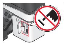
**Warning—Potential Damage:** Do not touch any cables, any network adapter, any connector, the memory device, or the printer in the areas shown while actively printing, reading, or writing from the memory card. A loss of data can occur.
