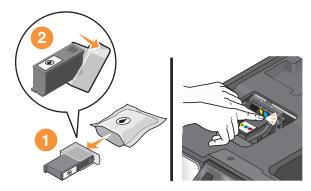
**Note:** Install the new ink cartridges immediately after removing the protective cap to avoid exposing the ink to air.
