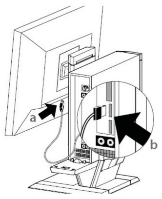
**7 a** Connect the monitor power cord to the monitor.
