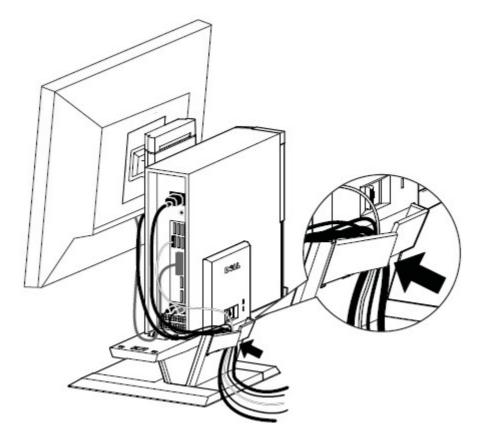
**11** Slide the cable cover over and down to attach it to the computer chassis.
