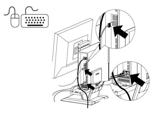
**10** Route the cables and power cords through the clip at the back of the AIO stand.
