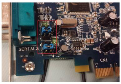
The serial add-in-card has two selectable jumpers:
