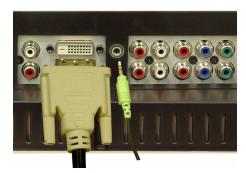
A digital signal that can support digital and convert analog to digital. DVI can be used for high resolution display and can support resolutions up to 1280 x 768.
