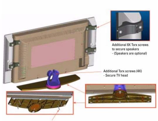
4X non-headed, T10, M5 threaded screw to bottom of TV stand base
