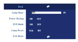
**LAMP HOUR**—Display the operating hours since the lamp timer reset.
