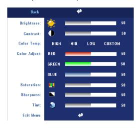
CONTRAST—Use — and ⊕ to control the degree of difference between the brightest and darkest parts of the picture. Adjusting the contrast changes the amount of black and white in the image.
