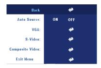
AUTO SOURCE—Select ON (the default) to autodetect the available input signals. When the projector is on and you press SOURCE, it automatically finds the next available input signal. Select OFF to lock the current input signal. When OFF is selected and you press SOURCE, you select which input signal you want to use.
