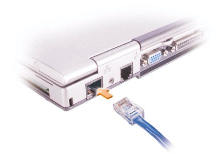
If you are connecting your computer to a network, connect the network cable to the network connector.
