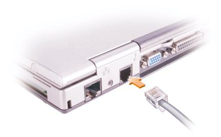
To use the modem, connect the telephone cable to the internal modem connector on the back of the computer.
