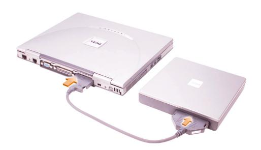
Connect the media bay cable to the external media bay and to the external media bay connector on the back of the computer.
