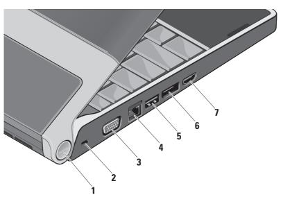
1 Power light – Illuminates when the computer is powered on. The different lights indicate the following:
