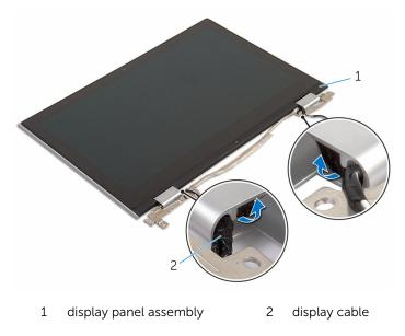
2 Using a plastic scribe, pry the display-panel assembly off the display back-cover and antenna assembly.
