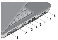
1 Air vents – The computer uses an internal fan to create airflow through the vents, which prevents the computer from overheating. The fan automatically turns on when the computer gets hot. Fan noise is normal and does not indicate a problem with the fan or the computer.
