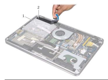
1 optical-drive assembly 2 mylar
