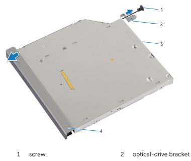
3 optical drive 4 optical-drive bezel
