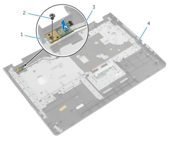
1power-button board2screw3power-button board cable4palm rest
