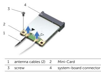
**3** Lift the Mini-Card out of the system-board connector.
