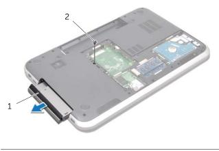
1 optical-drive assembly 2 screw
