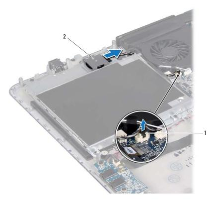
l coin-cell-battery cable connector 2 coin-cell battery
