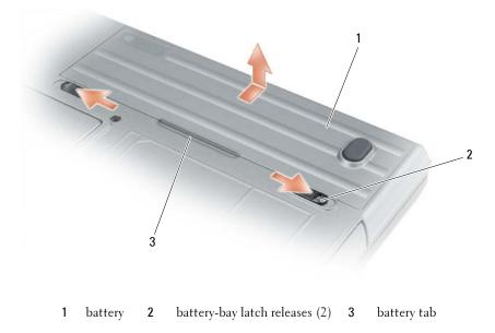
To replace the battery, follow the removal procedure in reverse order.
