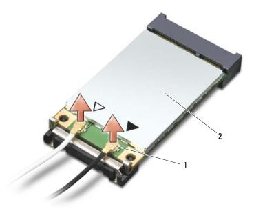
1 antenna cable connectors (2) 2 WLAN card
