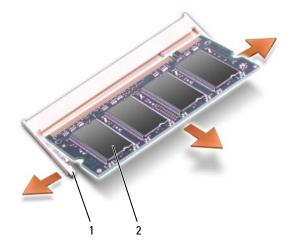
1 securing clips (2 per connector) 2 memory module
