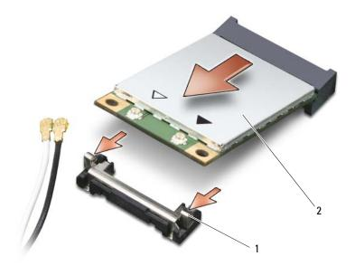
1 metal securing tabs (2) 2 WLAN card
