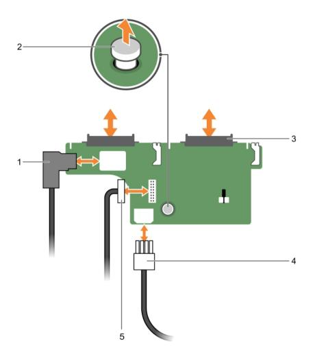
Figure 58. Removing and installing the optional 2.5 inch (x2) hard-drive backplane
