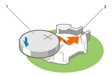
Figure 44. Installing the system battery
