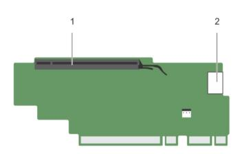
Figure 40. Identifying connectors on the expansion card riser 3 (alternate)
