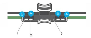
Figure 4. HDD indicators on the hard-drive tray backplane
