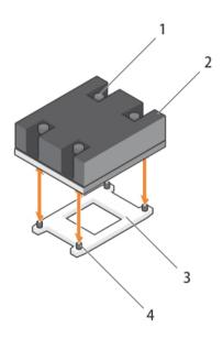
Figure 23. Removing and installing a processor heat sink
