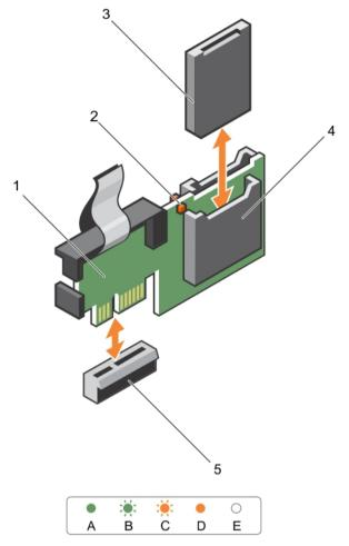
Figure 41. Removing and installing the Internal Dual SD Module (IDSDM)
