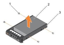
Figure 54. Removing and installing a hard drive into a hard-drive carrier
