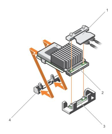
Figure 30. Removing and installing the integrated storage controller card
