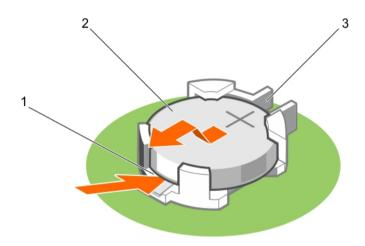
Figure 43. Removing the system battery
