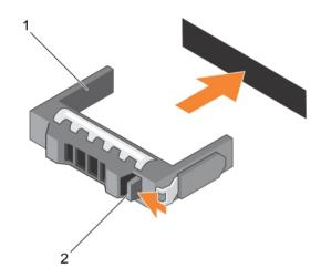
Figure 52. Removing and installing a 3.5 inch hard-drive blank
