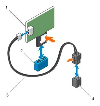
Figure 20. Removing and installing SATADOM
