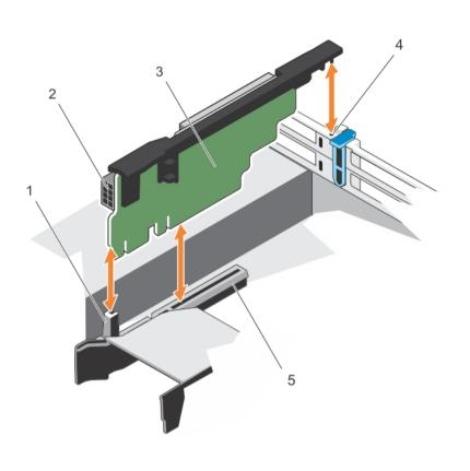
Figure 38. Removing and installing the expansion card riser 3
