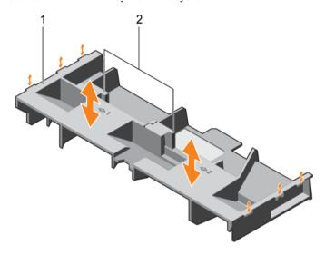
Figure 13. Removing and installing the cooling shroud
