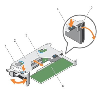
Figure 33. Removing and installing an expansion-card from expansion-card riser 1
