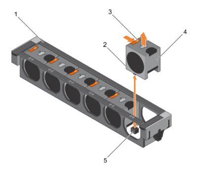
Figure 14. Removing and installing a cooling fan
