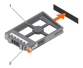
Figure 50. Removing and installing a 2.5 inch hard-drive blank
