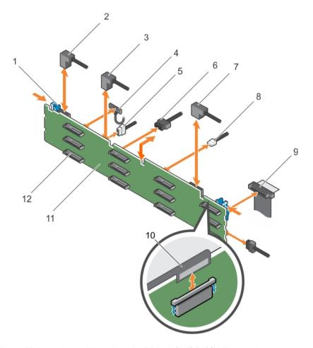
Figure 57. Removing and installing the 3.5 inch (x12) SAS/SATA backplane
