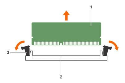
Figure 18. Removing and installing a memory module
