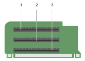
Figure 35. Identifying connectors on the expansion card riser 1
