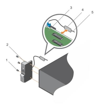
Figure 59. Removing and installing the control panel
