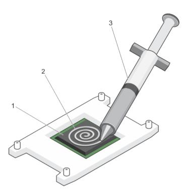
Figure 26. Applying thermal grease on the top of the processor
