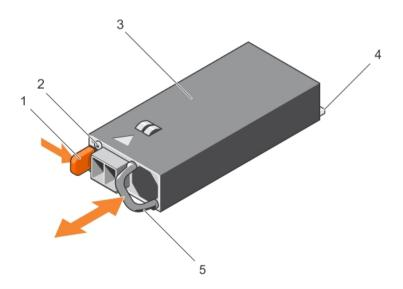
Figure 47. Removing and installing a DC power supply
