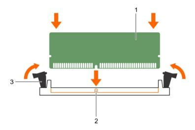
Figure 19. Installing the memory module
