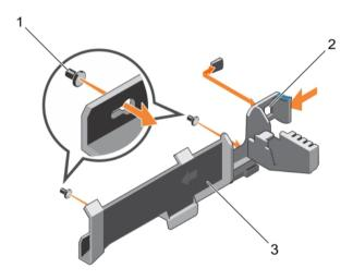
Figure 29. Removing and installing the cable retention bracket
