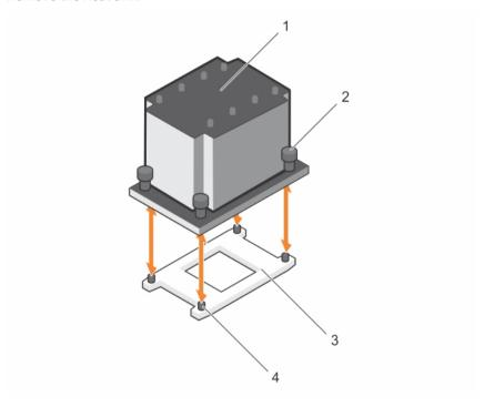
Figure 21. Removing and installing a processor
