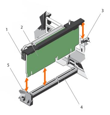
Figure 36. Removing and installing the expansion card riser 2
