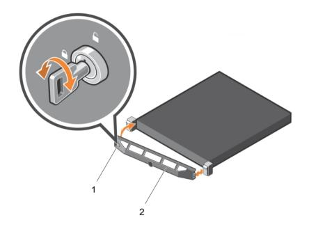
Figure 10. Removing and installing the front bezel
