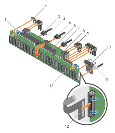
Figure 55. Removing and installing the 2.5 inch (x24) SAS/SATA backplane
