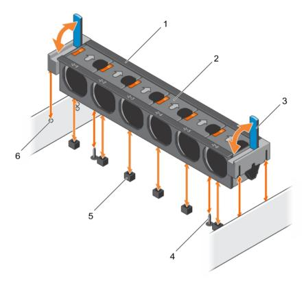
Figure 15. Removing and installing the cooling-fan assembly
