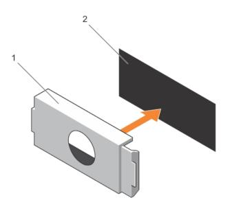
Figure 45. Removing and installing the power supply blank
