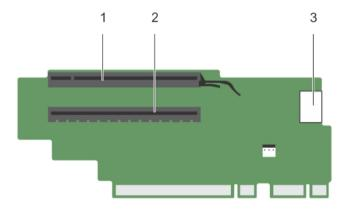
Figure 39. Identifying connectors on the expansion card riser 3 (default)
