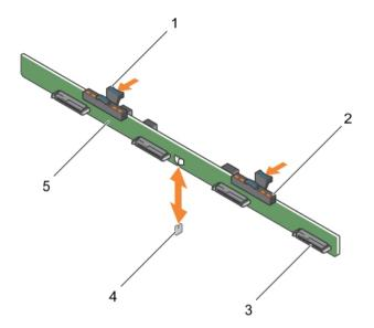
Figure 61. Removing and installing the 3.5 inch (x4) hard-drive backplane
