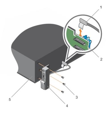
Figure 60. Removing and installing the I/O panel
