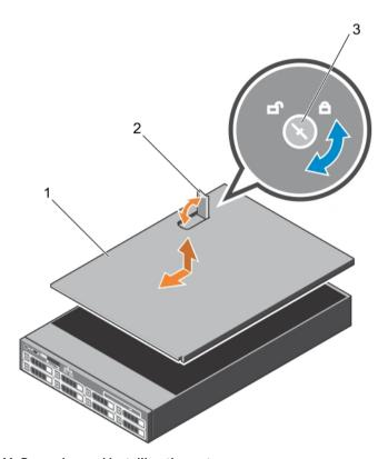
Figure 11. Removing and installing the system cover
