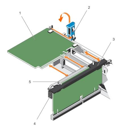
Figure 32. Removing and installing an expansion card from expansion-card riser 2 or 3
