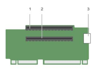
Figure 37. Identifying connectors on the expansion card riser 2
