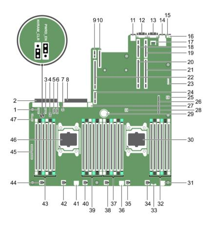
Figure 62. System board jumpers and connectors
