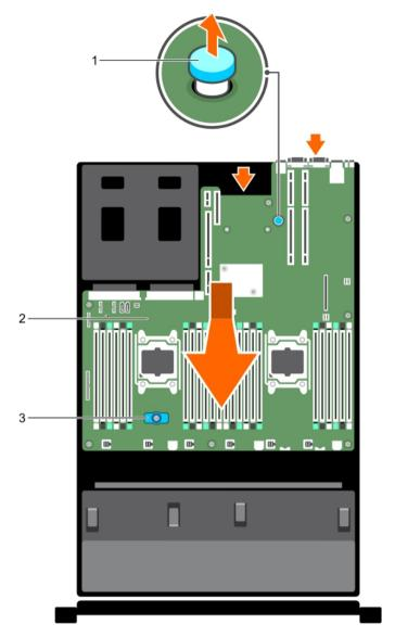
Figure 48. Removing and installing the system board
