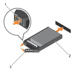
Figure 53. Removing and installing a hot-swap hard drive
