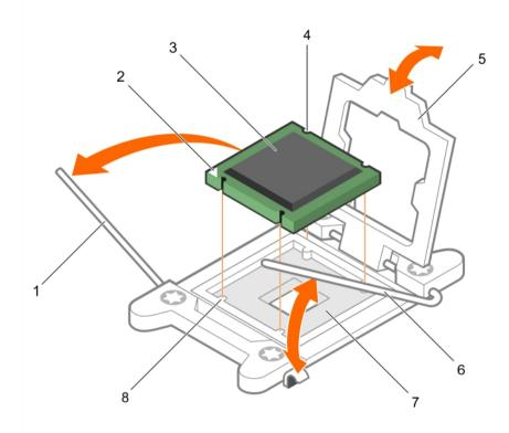
Figure 25. Removing and installing a processor
