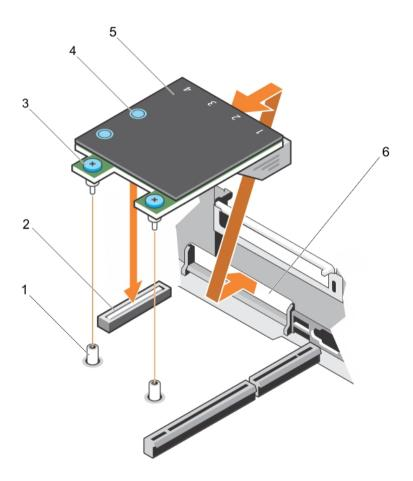
Figure 42. Removing and installing the Network Daughter Card (NDC)
