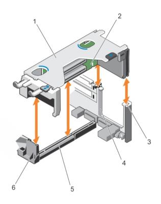
Figure 34. Removing and installing the expansion card riser 1
