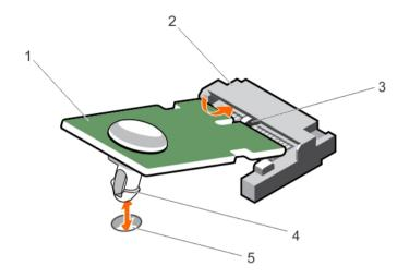
Figure 49. Installing the TPM
