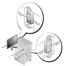
• If your computer is installed in a corner on a desk or under a desk, leave at least 5.1-cm (2-in) clearance from the back of the computer to the wall to permit the airflow required for proper ventilation.
