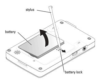
NOTE: Your Service Tag is located underneath the battery. You need your Service Tag if you access Dell Support at support.dell.com or if you call Dell for customer service or technical support.
