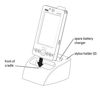
4 Align the connector on the bottom of the device with the connector on the cradle, and, keeping the front of the device flush with the front of the cradle, lower the device onto the cradle.
