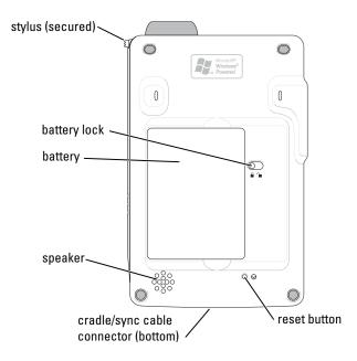
**BATTERY LOCK**—Use this switch to release and remove the main battery. See "Installing and Removing the Battery" on page 21.
