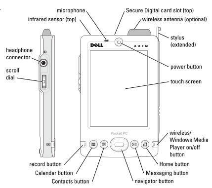
INFRARED SENSOR—The infrared sensor lets you transfer files from your device to another infrared-compatible device without using cable connections.
