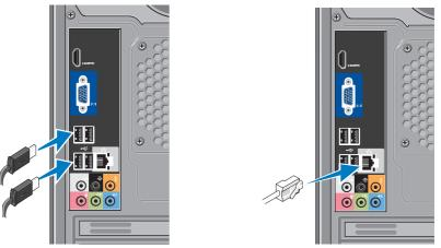
A network connection is not required to complete your computer setup, but if you have an existing network or Internet connection that uses a cable connection (such as a home cable modem or Ethernet jack), you can connect it now. Use only an Ethernet cable (RJ45 connector). Do not plug a telephone cable (RJ11 connector) into the network connector.
