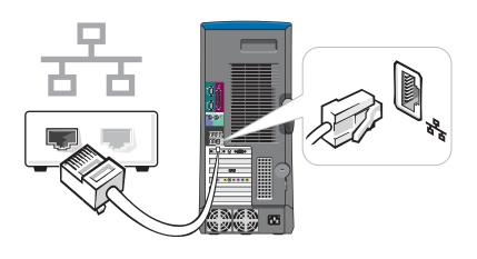
**If you have a network device**Connect a network cable to the network connector.
