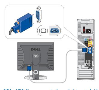
VGA→VGA: If your computer has only integrated video, use that connector. VGA→VGA: 如果您的计算机只有集成视频,请使用集成视频连接器。
