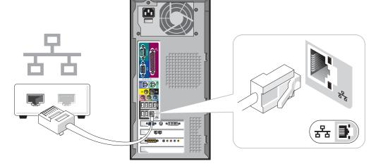
If you have a network device, connect a network cable (not included) to the network connector.
