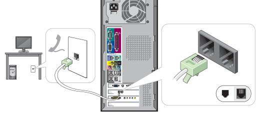
If you have a modem, connect a telephone cable to either of the modem connectors.
