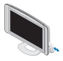
Insert the disc, with the label facing outwards and gently push the disc into the slot. The drive will automatically pull the disc in and begin reading its content. To eject a disc from the drive, gently touch the eject control.
