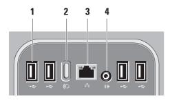
1 USB 2.0 connectors (4) — Connects to USB devices, such as a mouse, keyboard, printer, external drive, or MP3 player.
