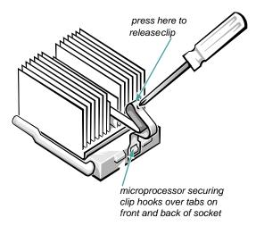
Figure 7-8. Microprocessor Securing Clip
