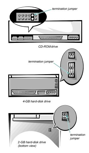
Figure 9-1. SCSI Termination Jumper Locations
