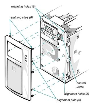
Figure 6-2. Removing the Front Bezel
