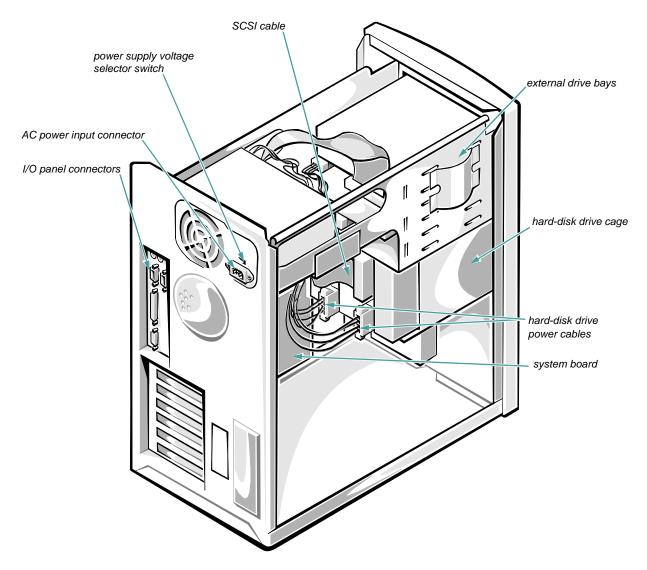
Figure 6-4. Inside the Chassis—Back/Left Side View
