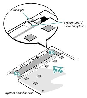
Figure 6-6. Replacing the System Board Assembly
