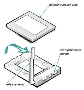
Figure 7-9. Removing the Microprocessor
