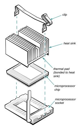
Figure 7-12. Installing the Heat Sink
