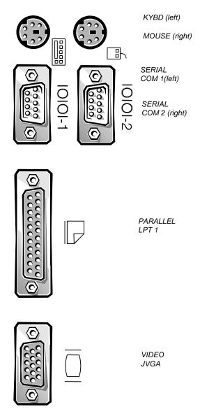
Figure B-2. I/O Ports and Connectors
