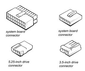
Figure 8-6. DC Power Cable Connectors
