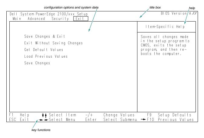
Figure 4-5. Exit Menu of the System Setup Program
