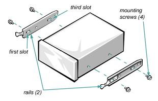
Figure 8-9. Attaching Drive Rails
