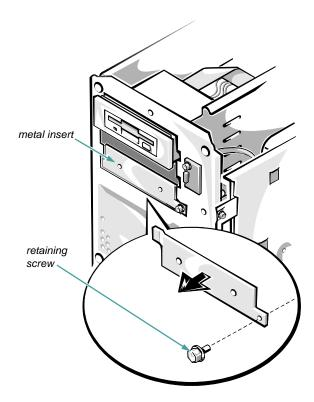
Figure 8-3. Removing a Metal Insert
