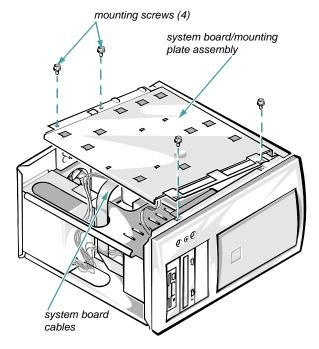
Figure 6-5. Removing the System Board Assembly
