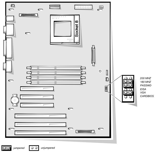
Figure B-1. System Board Jumpers
