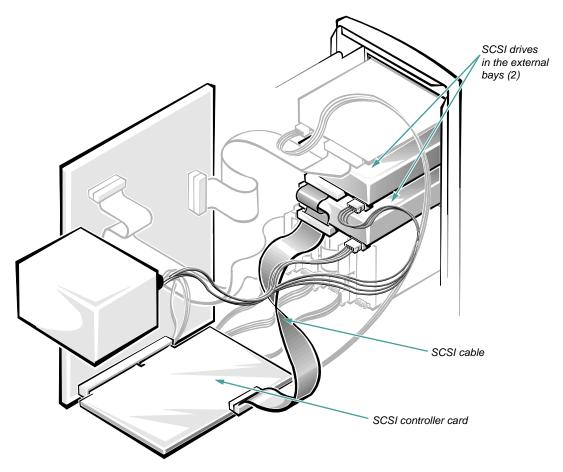
Figure 8-11. Connecting an Optional SCSI Controller Card
