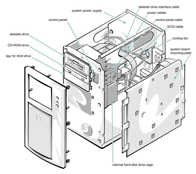
Figure 6-3. Inside the Chassis—Front/Right Side View
