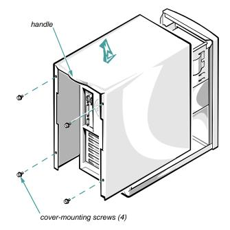
Figure 6-1. Removing the Computer Cover
