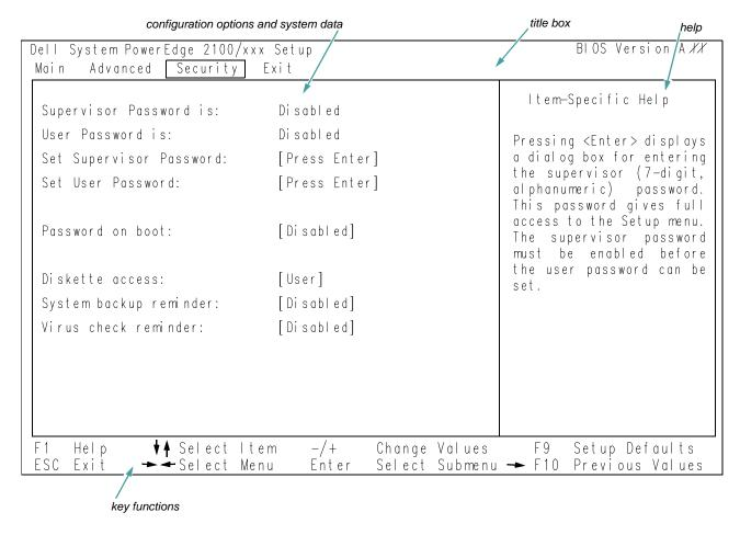
Figure 4-4. Security Menu of the System Setup Program
