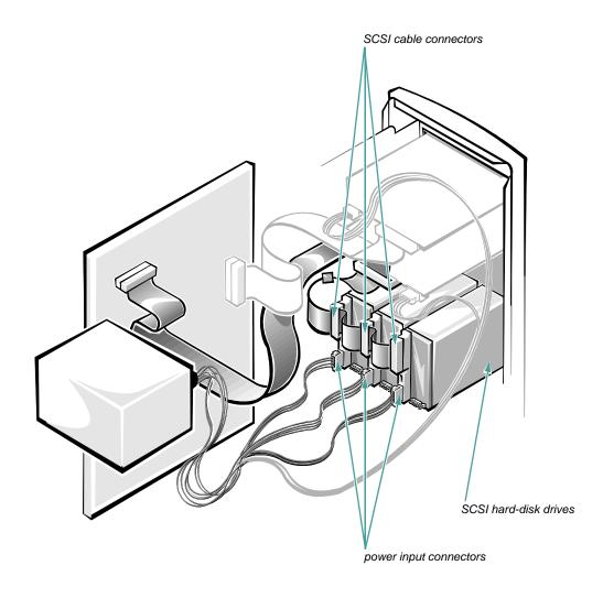
Figure 9-3. SCSI Cable for a PowerEdge 2100 System
