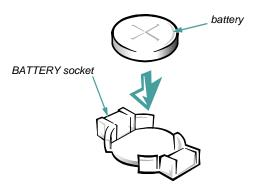
Figure 7-13. System Battery and Battery Socket
