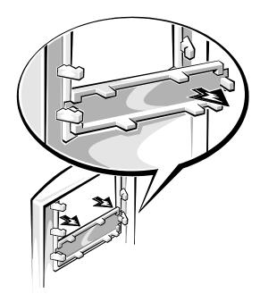
Figure 8-2. Removing a Plastic Insert
