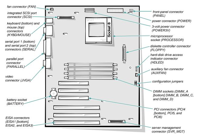
Figure 7-1. System Board Features
