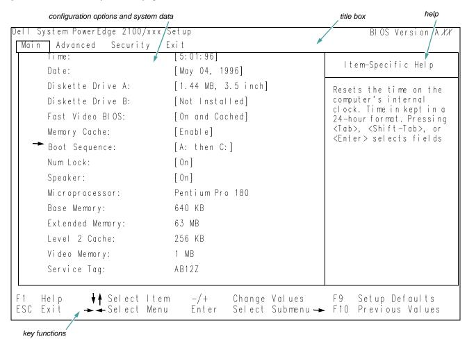
Figure 4-1. Main Menu of the System Setup Program
