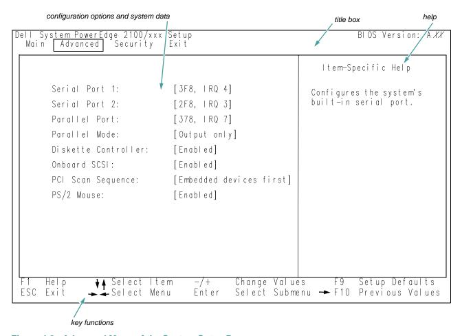
Figure 4-3. Advanced Menu of the System Setup Program
