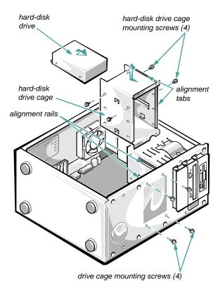
Figure 9-4. Removing the Hard-Disk Drive Cage
