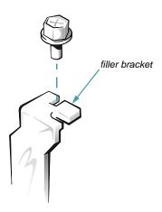
Figure 7-3. Removing the Filler Bracket
