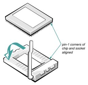
Figure 7-11. Installing the Microprocessor Chip
