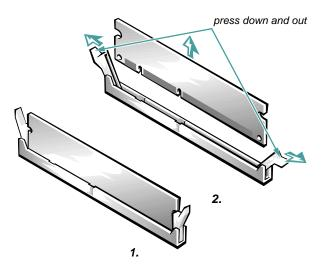
Figure 7-7. Removing a DIMM
