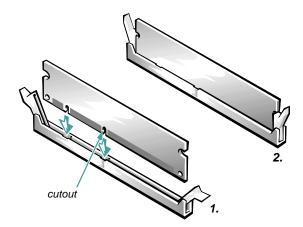
Figure 7-6. Installing a DIMM
