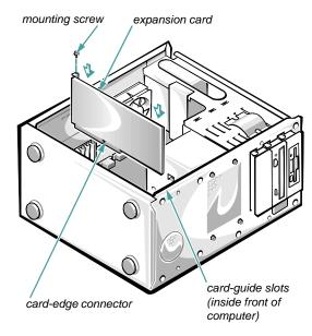
Figure 7-4. Installing an Expansion Card
