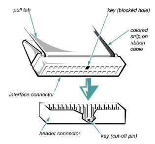
Figure 8-5. Header Connector
