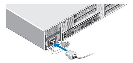
**6** Attach the power cable retention bracket on the right bend of the power supply handle. Bend the power cable into a loop as shown in the illustration and attach the cable to the bracket's cable clasp.
