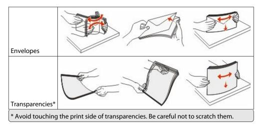
**5** Load the paper or specialty media. Slide the stack gently into the multipurpose feeder until it comes to a stop.
