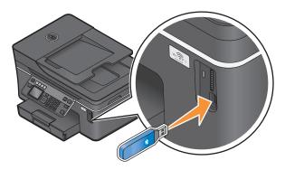
Bluetooth Dongle Connected appears on the display.
