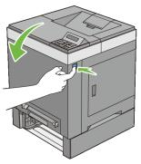
5 Open the belt unit until it stops and remove the jammed paper. Confirm that there are no scraps of paper remaining inside the printer.
