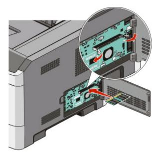
**6** Push the memory card into the connector until the latches *snap* into place. It may require some force to fully seat the card.
