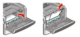
**Note:** If the paper is not easy to remove, then open the rear door to remove the paper.
