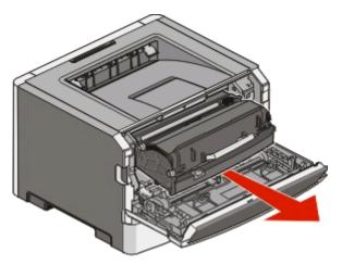
**Warning—Potential Damage:** Do not touch the photoconductor on the underside of the photoconductor kit. Use the cartridge handle whenever you are holding the cartridge.
