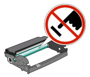
**5** Insert the toner cartridge into the photoconductor kit by aligning the rollers on the toner cartridge with the tracks. Push the toner cartridge in until it *clicks* into place.
