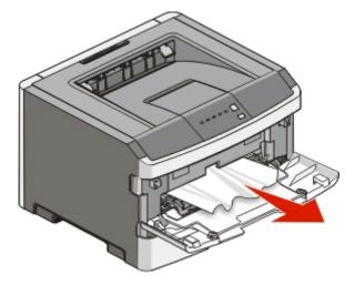
Paper jammed in the manual feeder can usually be grasped and pulled straight out. If the jam cannot be removed this way, check for jammed paper behind the photoconductor kit and toner cartridge unit. For more information, see "Clearing jams behind the photoconductor kit and toner cartridge" on page 102.
