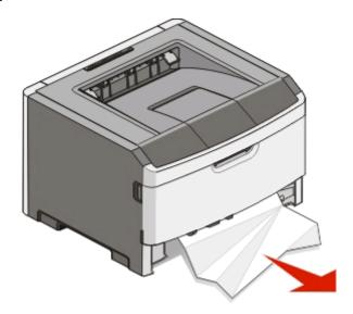
**3** If necessary, depress the lever to free the paper and remove the jam.
