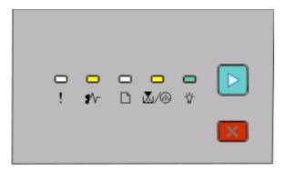
Remove the jam from the manual feeder.
