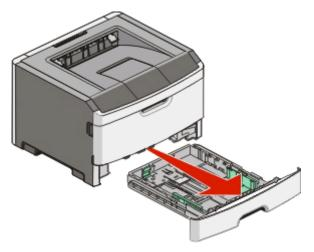
Do not remove trays while a job prints or when the Busy light sequence appears on the printer control panel. Doing so may cause a jam.
