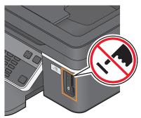
**Warning—Potential Damage:** Do not touch any cables, any network adapter, any connector, the memory device, or the printer in the areas shown while actively printing, reading, or writing from the memory card. A loss of data can occur.
