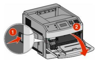
**2** Push the release latch, and then open the front cover.
