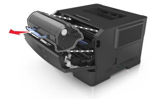
**3** Lift the blue handle, and then pull the imaging unit out of the printer.
