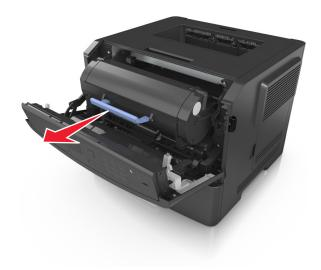
**3** Lift the blue handle, and then pull the imaging unit out of the printer.
