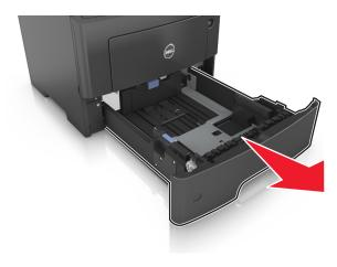
2 Squeeze, and then slide the width guide tab to the correct position for the size of the paper you are loading.
