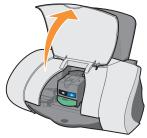
The ink cartridge carrier moves and stops at the loading position unless the printer is busy.
