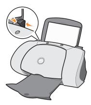
**NOTE:** To avoid smearing ink, remove each transparency or photo from the paper exit tray before the next one exits the printer. Transparencies and photos may require up to 15 minutes to dry.
