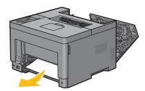
**7** Insert trayl into the printer, and push until it stops.
