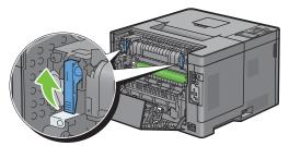
3 If the document is jammed under the fusing unit, remove the jammed document from under the fusing unit.
