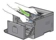
4 To remove the toner cartridge from the old drum cartridge, grasp the toner cartridge lock lever, and then raise it upward to unlock.
