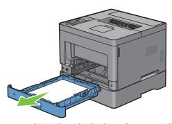
**5** Pull the optional 550-sheet feeder from the printer about 200 mm.
