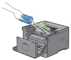
**7** Grasp the toner cartridge lock lever, and then pull it down until it stops.
