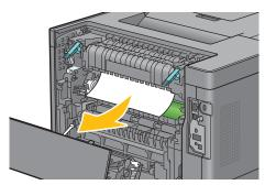
4 If the document is jammed above the fusing unit, raise the tab of the inner part, and turn it to open.
