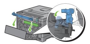
4 Make sure that the arrow marks on the Transfer Unit and the printer face each other, and then press the two tabs on Transfer Unit inward to lock.
