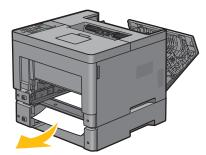
Insert the optional 550-sheet feeder into the printer, and push until it stops.
