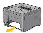
**6** Insert trayl into the printer, and push until it stops.
