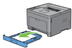
**NOTE:** Be sure to remove all the paper from tray1 before removing the retard roller.
