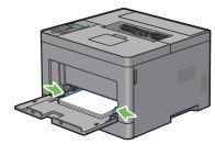
5 On the operator panel, press the ∨ or ∧ button until the desired paper size is highlighted, and then press the ✓ (Set) button.
