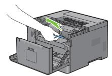
**3** Hold both sides of the drum cartridge with your hands, and then pull it out completely.
