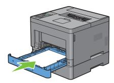
**10** Insert the MPF into the printer, push until it stops, and close the MPF.
