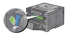
**3** Slide the envelope switches on the both sides of the fusing unit to the position.
