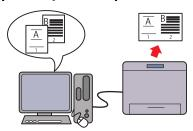
The Multiple Up feature enables you to print documents as reduced-size documents containing multiple pages on a single sheet of paper by setting from the printer driver. This feature helps save paper.
