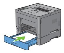
**9** Insert trayl into the printer, and push until it stops.
