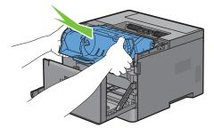
**3** Grasp the handle on the front of the drum cartridge, and then push and install the drum cartridge until it stops.
