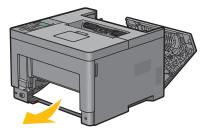
Insert trayl into the printer, and push until it stops.
