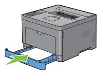
**NOTE:** If the front side of the tray is extended, the tray protrudes when it is inserted into the printer.
