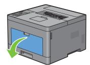
**5** Grasp both sides of the MPF, and then pull the MPF from the printer.
