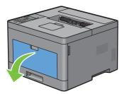
**2** Grasp both sides of the MPF, and then pull the MPF from the printer.
