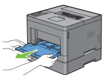
**4** Pull the tray 1 out of the printer about 200 mm.
