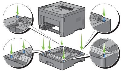
**9** Secure the optional 550-sheet feeder to the printer by tightening the two screws provided with the feeder, using a coin or similar object.
