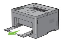
**2** Grasp both sides of the MPF, and then pull it out of the printer.
