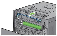
7 Press down the levers on both sides of the fusing unit.
