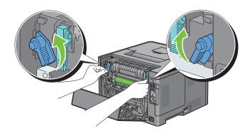
4 Grasp the grips on both sides of the fusing unit placing thumb on the knurling, and then pull out the unit.
