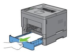
**6** Hold the optional 550-sheet feeder with both hands, and remove it from the printer.
