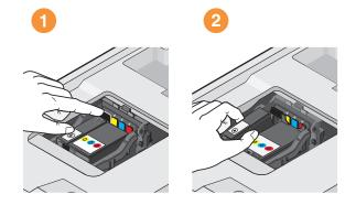
Note: Do not reinstall used ink cartridges once you remove them from the printhead.
