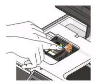
**Note:** Install the new ink cartridges immediately after removing the protective cap to avoid exposing the ink to air.
