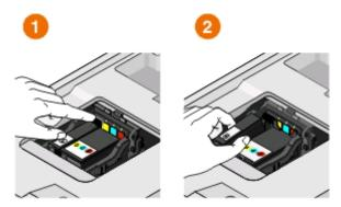
**Warning—Potential Damage:** Do not remove the old cartridges until you have the new cartridges available, or the ink remaining in the printhead may dry out and clog the nozzles.
