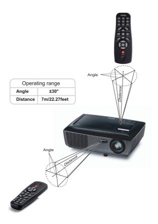
**NOTE:** Actual operating range may slightly differ from the diagram. Weak batteries will also prevent the remote control from properly operating the projector.
