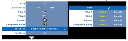
**VGA-A**—Use **<** and **≥** to enable or disable VGA-A input.
