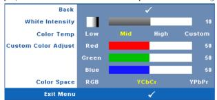
**WHITE INTENSITY**—Use  $\triangleleft$  and  $\triangleright$  to adjust the display white intensity.
