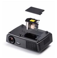
9 Reset the lamp usage time by selecting "Yes" for Lamp Reset in the OSD Lamp tab (see Lamp menu on page 34). When a new lamp module has been changed, the projector will automatically detect and reset the lamp hours.
