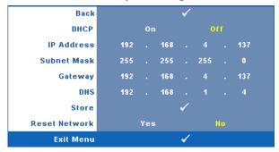
**DHCP**—If a DHCP server exists in the network to which the projector is connected, the IP address will automatically be acquired when you select DHCP On. If DHCP is Off, manually set the IP Address, Subnet Mask, and Gateway. Use to select the number of IP Address, Subnet Mask, and Gateway. Key in Enter to confirm each number and then use \( \) to set the next item.
