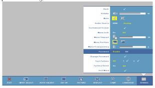
28 Using Your Projector h Enable the Password function will pop-up a character screen, key in a 4digit number from the screen and press the Enter button.
