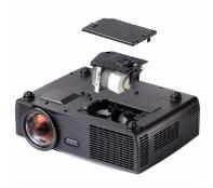
9 Reset the lamp usage time by selecting "Yes" for Lamp Reset in the OSD Lamp tab (see Lamp menu on page 41). When a new lamp module has been changed, the projector will automatically detect and reset the lamp hours.
