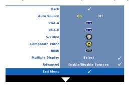
AUTO SOURCE—Select Off (the default) to lock the current input signal. If you press the Source button when the Auto Source mode is set to Off, you can manually select the input signal. Select On to auto detect the available input signals. If you press the Source button when the projector is on, it automatically finds the next available input signal.
