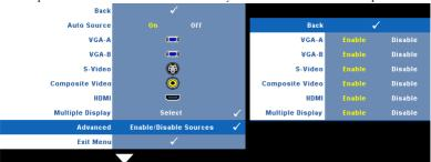
**VGA-A**—Use **<** and **>** to enable or disable VGA-A input.
