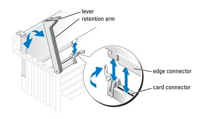
**5** Pull the securing tab (if present), grasp the card by its top corners, and ease it out of its connector.
