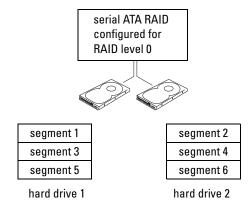
Another advantage of a RAID level 0 configuration is that it utilizes the full capacities of the drives. For example, if you have two 120-GB drives installed, you have 240 GB on which to store data.
