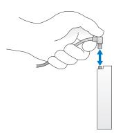
Most interface connectors are keyed for correct insertion; that is, a notch or a missing pin on one connector matches a tab or a filled-in hole on the other connector.
