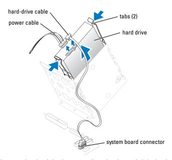
**4** Press the tabs on each side of the drive towards each other and slide the drive up and out.
