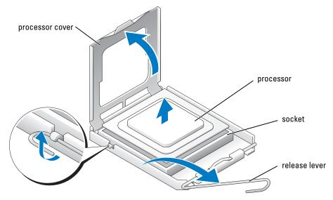
Remove the processor from the socket. Leave the release lever extended in the release position so that the socket is ready for the new processor.
