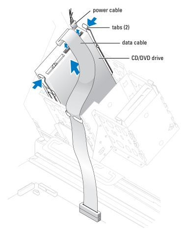
**3** Press inward on the two tabs on the sides of the drive, and then slide the drive upward and remove it from the drive bay.
