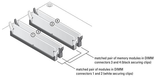
NOTICE: If you remove your original memory modules from the computer during a memory upgrade, keep them separate from any new modules that you may have, even if you purchased the new modules from Dell. If possible, do not pair an original memory module with a new memory module. Otherwise, your computer may not start properly. You should install your original memory modules in pairs either in DIMM connectors 1 and 2 or DIMM connectors 3 and 4.
