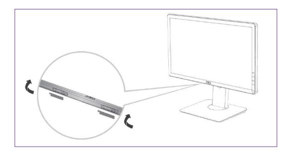
3. Connect the Soundbar to the Dell Monitor.
