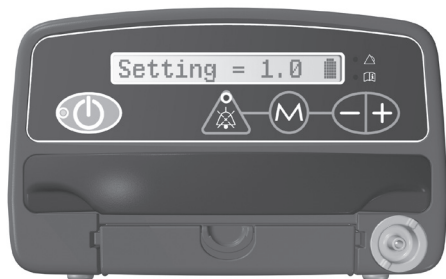
Figure 10. Concentrator operating on battery power.
