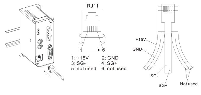
If the connection of PD-01 to VFD drives does not conform the table listed in page 2, users need to provide external 15VDC supply the power to PD-01 (not through the communication cable). Refer to the pin assignment of RJ11, it is allowed to supply power to PD-01 via RJ11.
