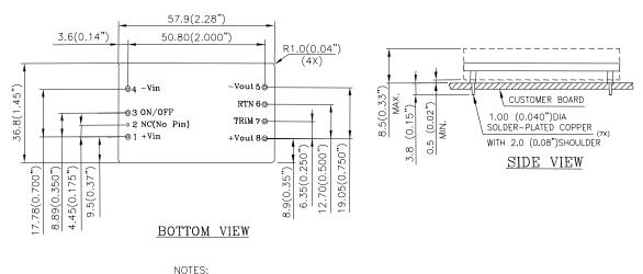
DIMENSIONS ARE IN MILLIMETERS AND (INCHES) TOLERANCES: X.Xmm±0.5mm(X.XX in.±0.02 in.) X.XXmm±0.25mm(X.XXX in.±0.010 in.) ON/OFF: NEGATIVE LOGIC ENABLE(OPEN=OFF,-Vin=ON)
