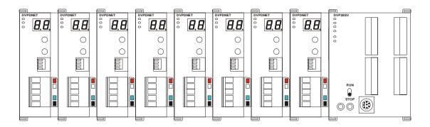
The index of DVPDNET-SL is its number. The first DVPDNET-SL on the left hand side of DVP-SV is No. 1, the following DVPDNET-SL modules are No.2, No.3, No.4 and so on.
