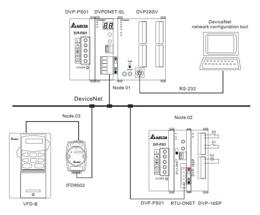
2. Set up DVPDNET-SL, DNA01 and RTU-DNET according to the table below.
