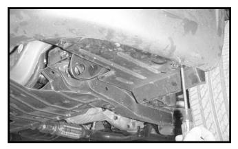
**8.** Remove two plastic push fasteners from each side underneath facia to inner wheel well extension.
