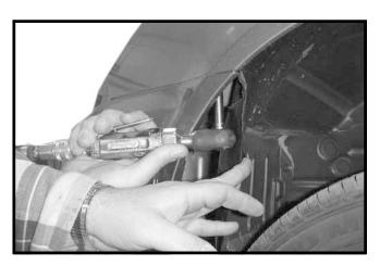
Pull inner wheel well extension away from fender to gain access to remove one screw, facia to fender, on each side.
