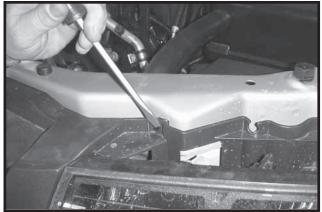
1. Open hood and release four plastic push fasteners from grill.
