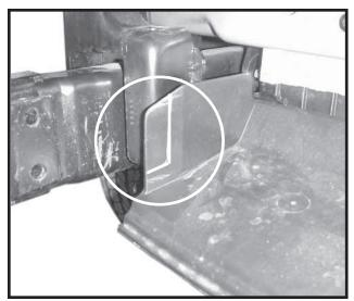
7. Notch plastic shield according to picture.
