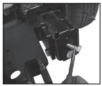
**9.** If drilling is needed insert shorter bolt using needle nose pliers as shown above.
