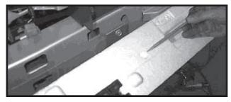
Push styrofoam against two bolt heads and cut out styrofoam for bolt head clearance. Attach styrofoam with two 1/4" x 1-1/2" sheetmetal screws and 1/4" flatwashers.
