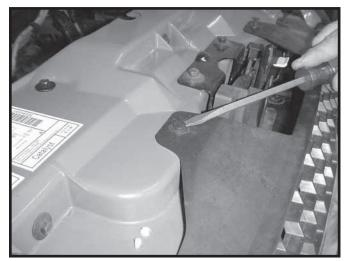
5. Remove grill, four plastic push fasteners, lift up and out. Remove two plastic push fasteners from top of facia and remove facia.
