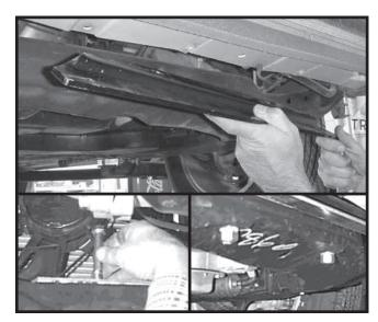
11. Attach narrow subframe mount with 1/2" x 4" bolts, lockwashers, and nuts on bottom side.
