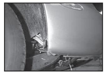
2. Remove inner fender to facia screw. Pull inner fender back or remove completely to gain access to one bolt, fender to facia. Do this on each side.
